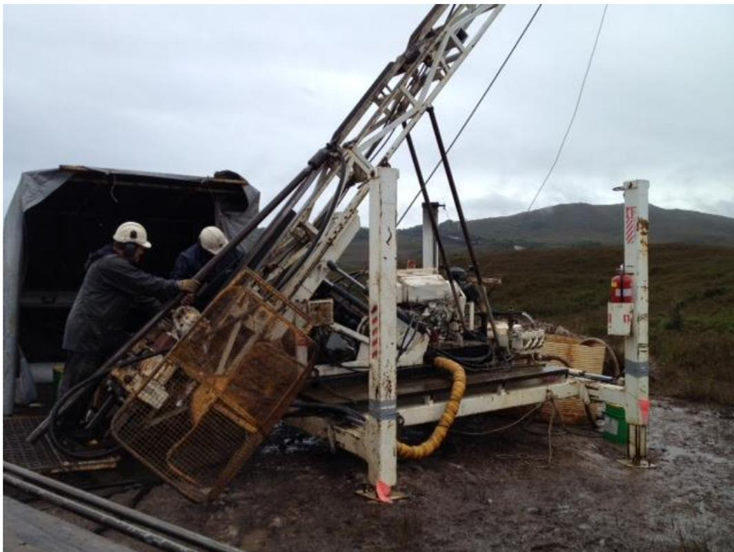
**Figure 3: Diamond Drilling at St Dizier**
