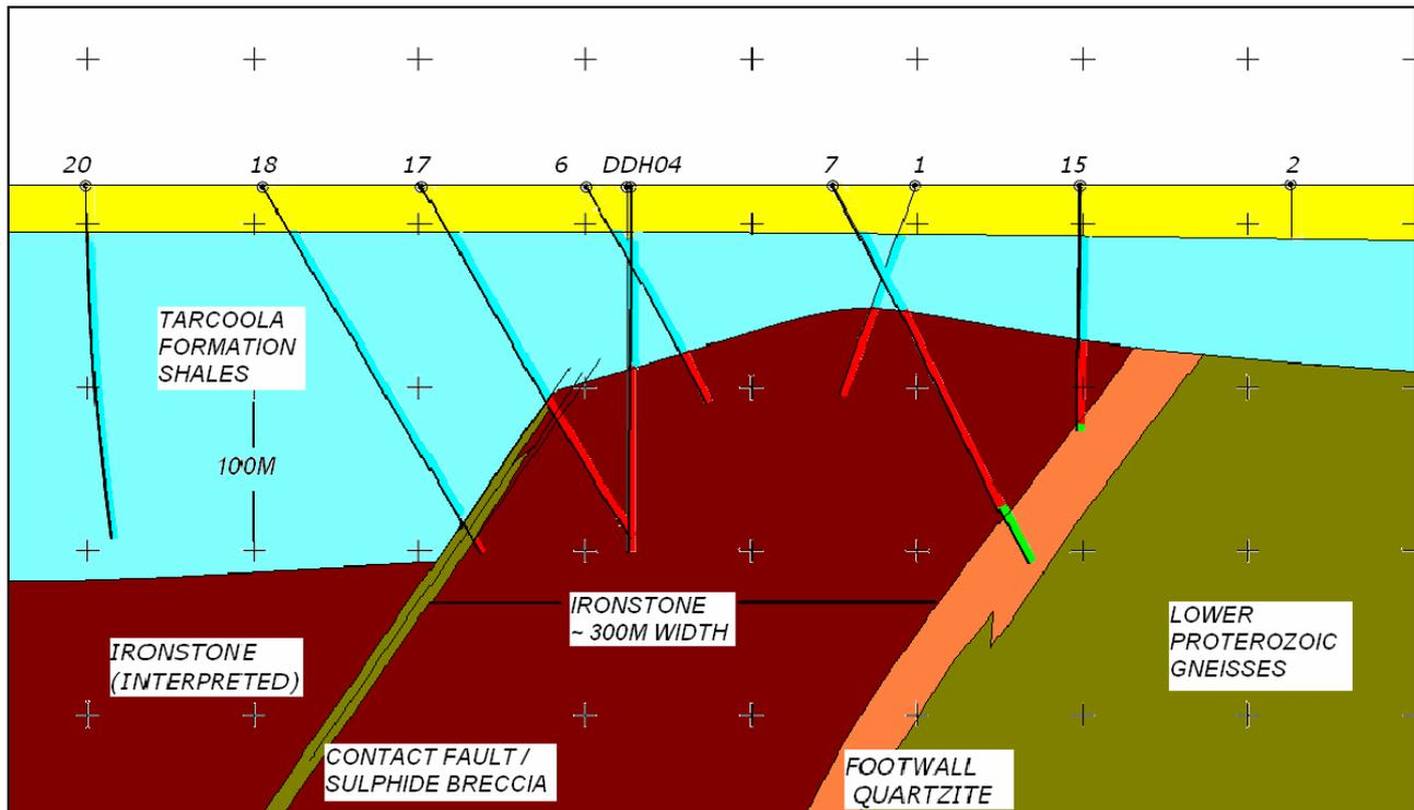
**Figure 2 – Interpretative geological section, southern section, Coolybring**
