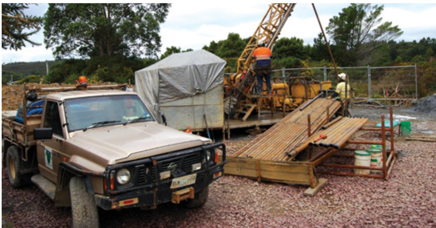
A second diamond rig at Severn carries out infill drilling on the current resource on the outskirts of Zeehan
