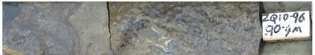
Core sample from interval 90-91m grading 3.5% tin – hole ZQ96
